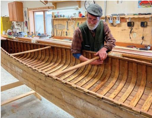
The boat in question is a 17 foot canoe made by the Shell Lake Boat Company sometime in the 1940s. It was in pretty rough shape when the Churchills acquired it. Restoration of the canoe to something suitable for a museum would require new outwales, spliced inwales, repairing and replacing decks, seats, keel and stems, and of course new canvas, paint, varnish, and fasteners throughout. It would be quite a project. The NMFSH asked the Wisconsin Canoe Heritage Museum (WCHM) for help.
