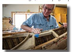
Most of the restoration work is being done by WCHM volunteers Jamie Dunn and Mike Johnson. All the broken ribs and planks have been replaced (including the ones with gunshot holes), and all the seats have been re-caned (all ten of them). Varnishing has begun but the decks still need to be fabricated. Soon
